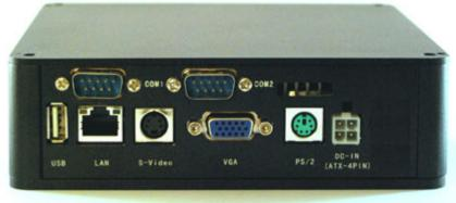
This MiniPC was especially designed for fleet applications. The Car-PC can be connected directly to the car battery (12V). Based on ignition plus, the PC will start and shutdown. The PC is offering several boot possibilities due to the internal connectors: 2.5" HDD or SSD, CompactFlash or USB.
